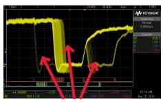
Infrequent glitches and signal jitter captured after 1 second on 3000 X-Series, D0 and D1 turned on with > 1,000,000 wfms/s.
